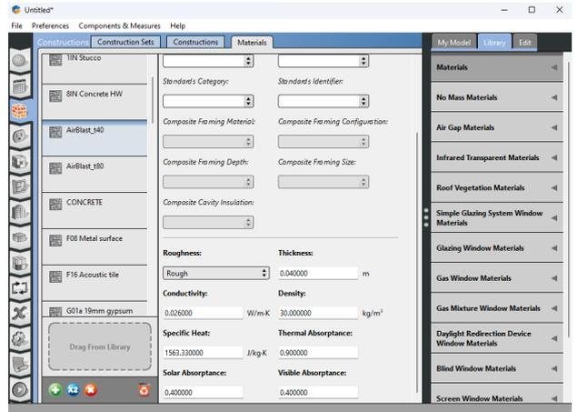
Fig. 5: Openstudio GUI. On the screenshot, we setup the “Airblast\_t40” material by modifying the material thickness, conductivity, etc.
