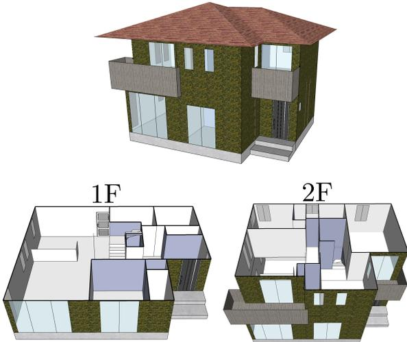
Fig. 3: High-fidelity 3D modeling of the house from the technical drawings of Fig. 2 using Sketchup. The lower left and right figures show the cross section of the first and second floors, respectively.
