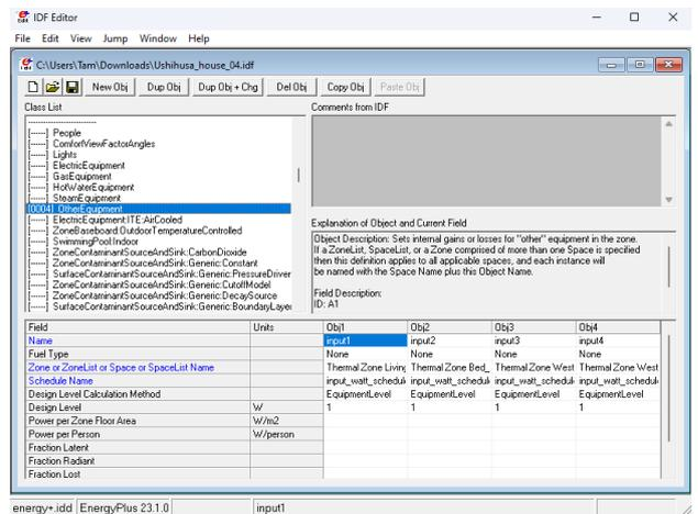
Fig. 6: EPLaunch IDF Editor. On the screenshot, we define and position the four HVACs, which are located in the living room (1F), the bedroom (2F), and the two western-style rooms (2F).
