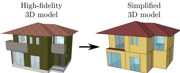
Fig. 4: Conversion from the high-fidelity model (left) to a simplified one (right), which must be eventually recognizable by EnergyPlus. Note that, since the balcony and the doors on the left are not recognized by EnergyPlus, they must be deleted in the simplified version on the right.
